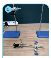
Using two clamp stands, clamps and bosses, fix the clamps at right angles to the clamp stand upright pole. Ensure both are at the same height. Set the stands 20-25cm apart.
