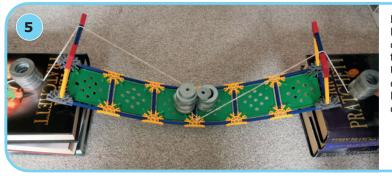
Remove the maximum load from the bridge. Bring one length of string over the upright on the right side of the bridge, and bring the other length over the upright on the left. Using some more of the small masses, weigh down the strings on either end of the bridge. Now return the original maximum load to the centre of the bridge. What do you notice?
