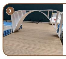
If vertical supports are to be added, tape the appropriate number of supports into position, parallel to the piers, and between the deck and arch strips. These should be symmetrical: if adding one each side, they should be as close to the same length and same position either side of the centre. If adding more than one support each side, they should be evenly spaced, and again symmetrical on both sides.
